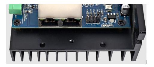
In the picture, at 1,2,3,4 positions, add a jumper cap to indicate 1, and no jumper cap to indicate 0.
