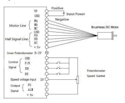
Note: If external potentiometer speed control is not required, SV and +5V can be directly shorted, and then controlled by shorting GND and EN for start/stop.
